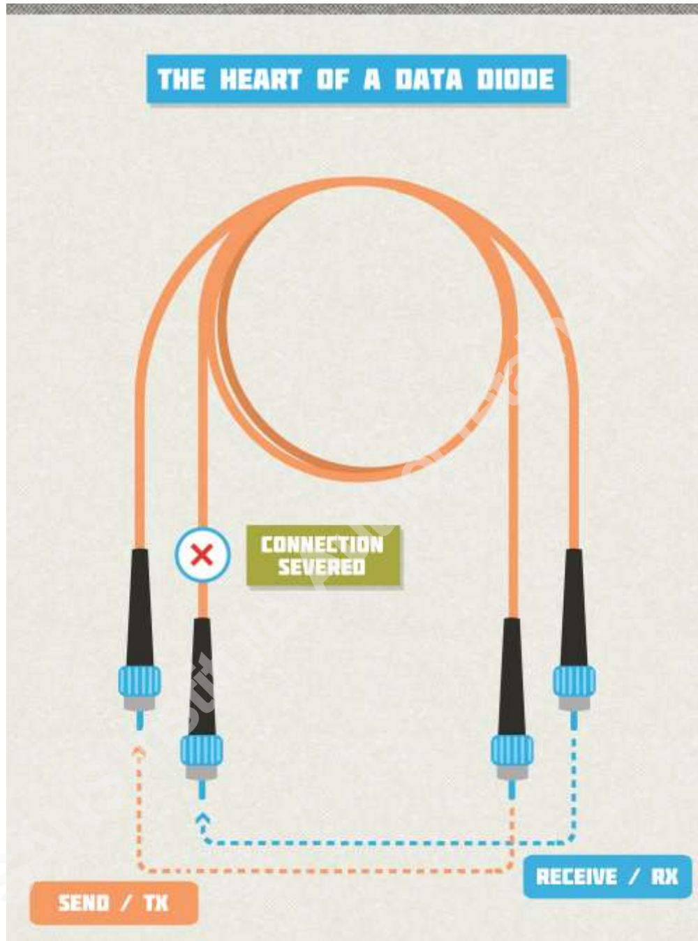
Figure 1 - Base Concept of a Data Diode.
